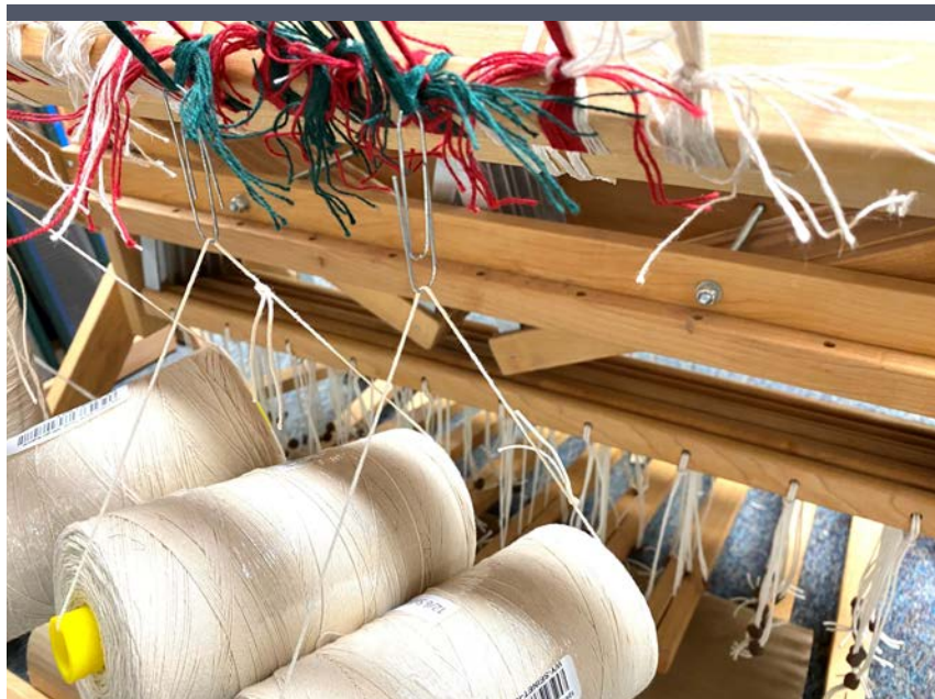
Tension problems caused by uneven take-up can be remedied. Warp-thread weights can be purchased or created from household items. Here we used paper clips and tubes of yarn for improvised weights.
