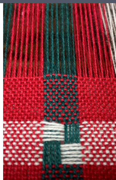
Some structures can cause tension problems, as shown here.
