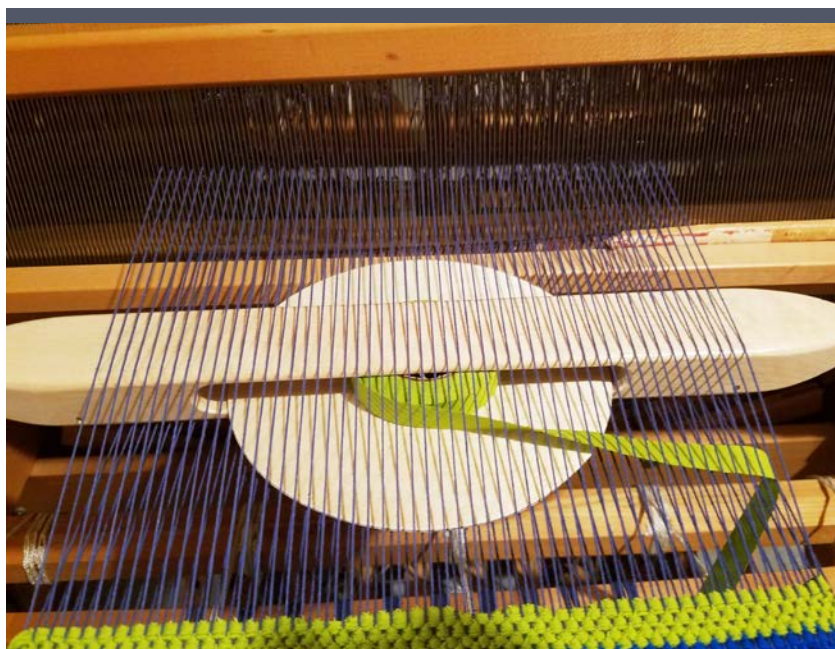
The width of the poppana disk dictates that you keep the fell line far enough from the reed to allow the shuttle enough room in the shed to pass.
