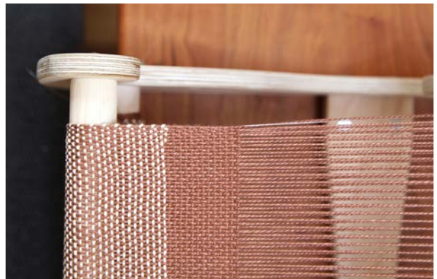
Fishing line sleyed alongside the selvage threads on each side of the loom helps to prevent too much draw-in.
