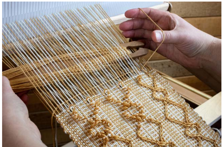
Pass the shuttle out of the warp and through a large loop to secure a chain.
