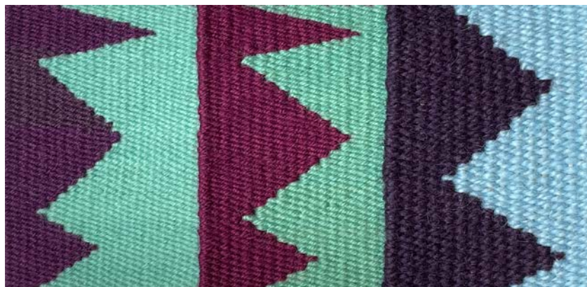
Three warp setts were used in these examples: left , 10 epi with 12/6 cotton seine twine; center , 8 epi with 12/9 cotton seine twine; and right , 6 epi with 12/18 cotton seine twine.
