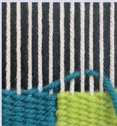
⑤ The blue-green weft is able to weave over the last pick of the yellow-green weft in the correct shed because both were set up to meet and separate.
