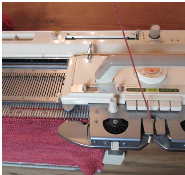
Keeping both the yarn tension and stitch-gauge tension loose, moving the carriage back and forth reveals the purl side.
