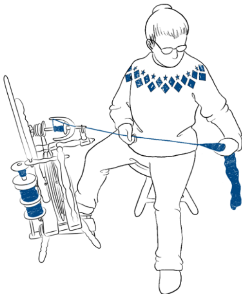
Figure 5. If the spinner places only one foot on a treadle and sits at an angle to the orifice, the shoulders are protected.
