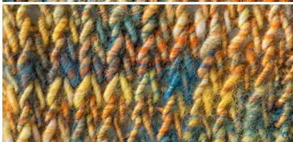
The colors in the mixed blend were more muted, which led to an optical blending effect. Spun samples with twist angles: (from top) 20 degrees, 40 degrees, and 60 degrees.
