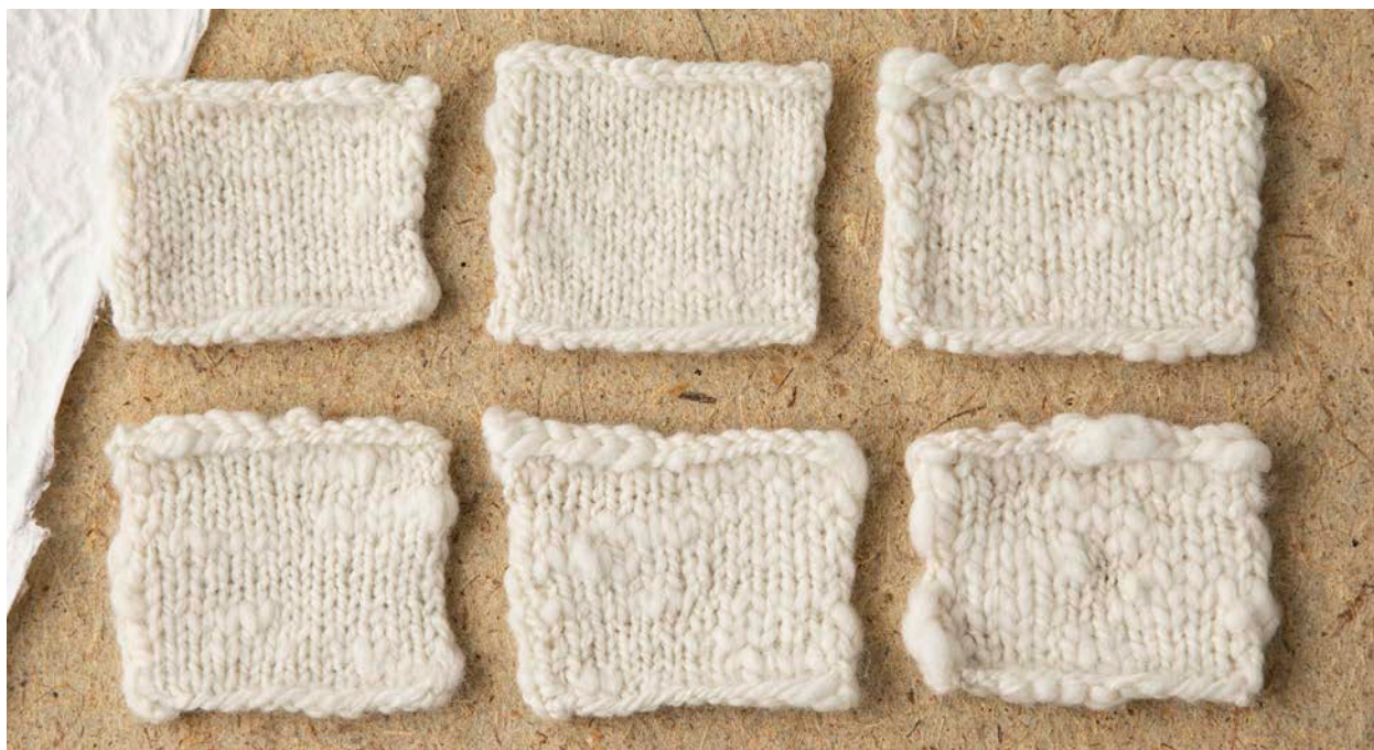
Knitted swatches from the second set of yarns, all made from one slub ply and one thin ply. Top row: small, spaced slubs; small, randomly spaced slubs; and small, back-to-back slubs. Bottom row: large, spaced slubs; large, randomly spaced slubs; and large, back-to-back slubs
