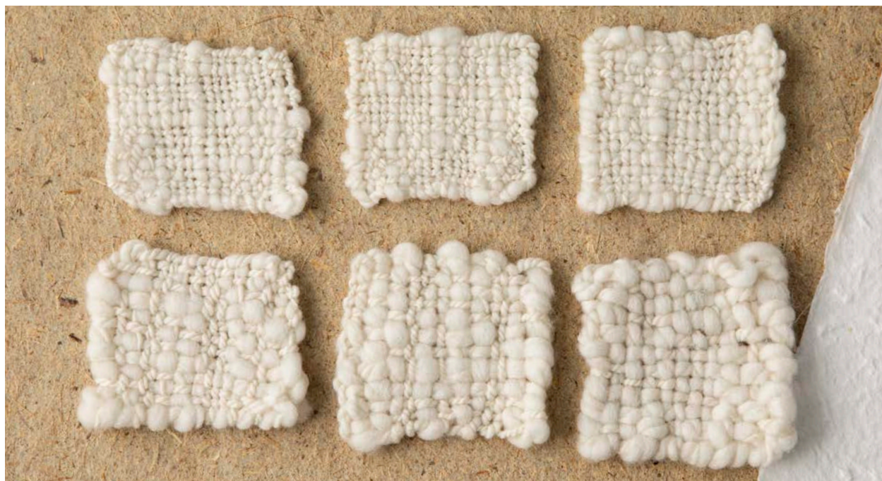
Woven swatches from the first set of yarns, two-ply yarns created with two slubbed singles. Top row: small, spaced slubs; small, randomly spaced slubs; and small, back-to-back slubs. Bottom row: large, spaced slubs; large, randomly spaced slubs; and large, back-to-back slubs
