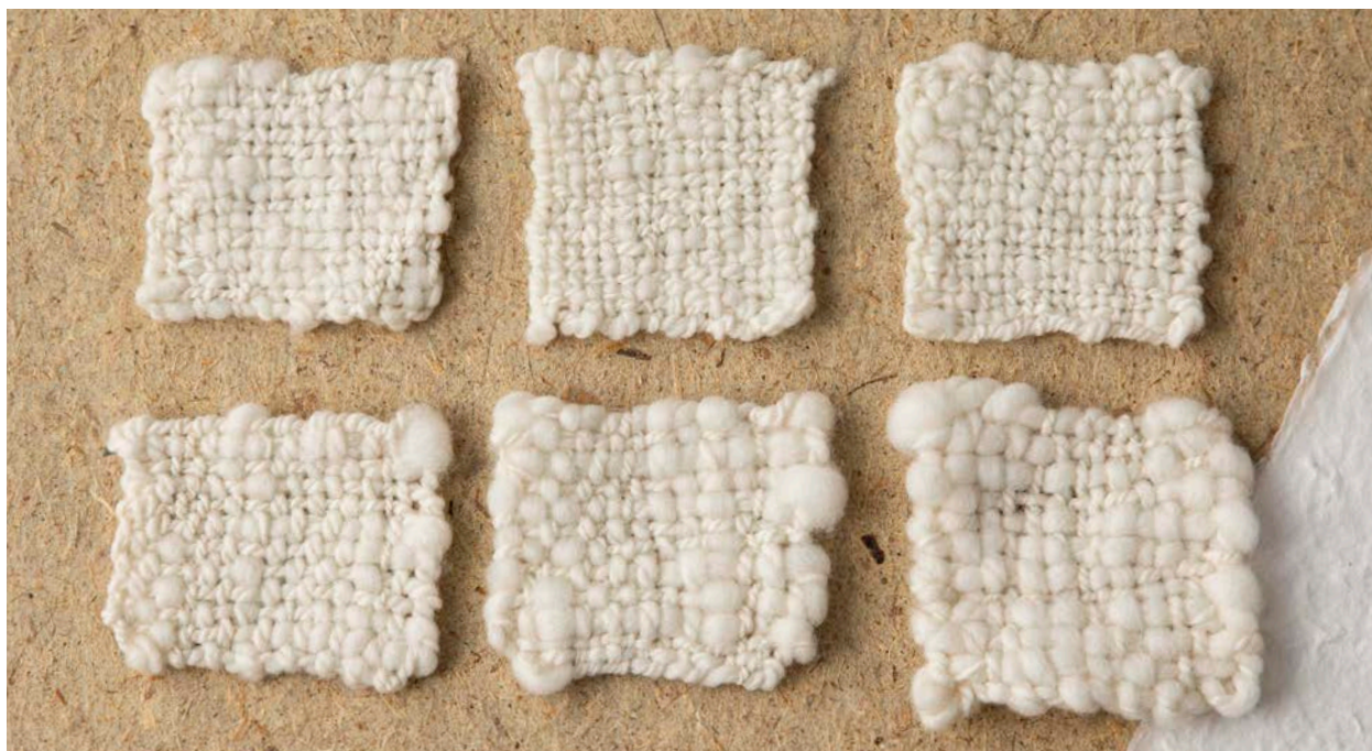
Woven swatches from the second set of yarns, all made from one slug ply and one thin ply. Top row: small, spaced slubs; small, randomly spaced slubs; and small, back-to-back slubs. Bottom row: large, spaced slubs; large, randomly spaced slubs; large, back-to-back slubs
